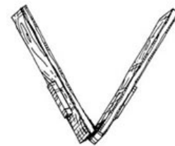
Figure 5. Construct a clapper by hinging together two, 24-inch 2 x 4s. Smack the two sides together. (Drawing by Jenifer Rees.)
