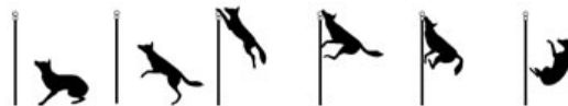
Figure 9. The "Coyote Roller" prevents coyotes from being able to get the foothold necessary to hoist them over a fence.
